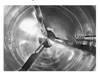
PerMix PDI series High Speed Mixer, also called Mixer Granulator, Wet Granulator, or High Shear Mixer Granulator, is an efficient and versatile blending machine for mixing of dry powders, or granulating with the addition of liquid binder, within a very short time and with excellent cleaning abilities. It is able to give perfect result for mixing due to the innovative design of a central Impeller type mixer with a side high speed Chopper.
